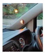
Mount the LED indicators on both A-pillars in the driver's field of vision. The displays are self-adhesive.
